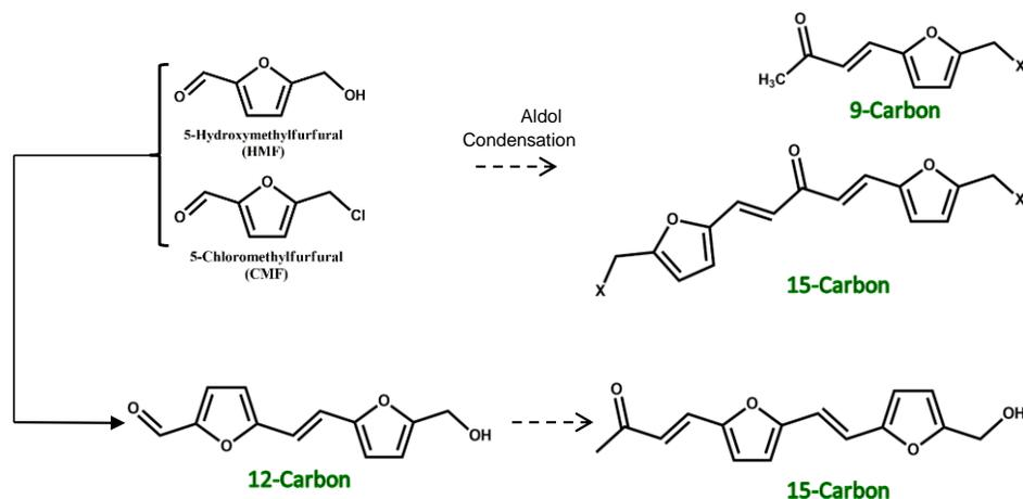
Figure 11. Biofuel precursors by Aldol condensation 9-, 12-, and 15-C Vinyl condensates.
