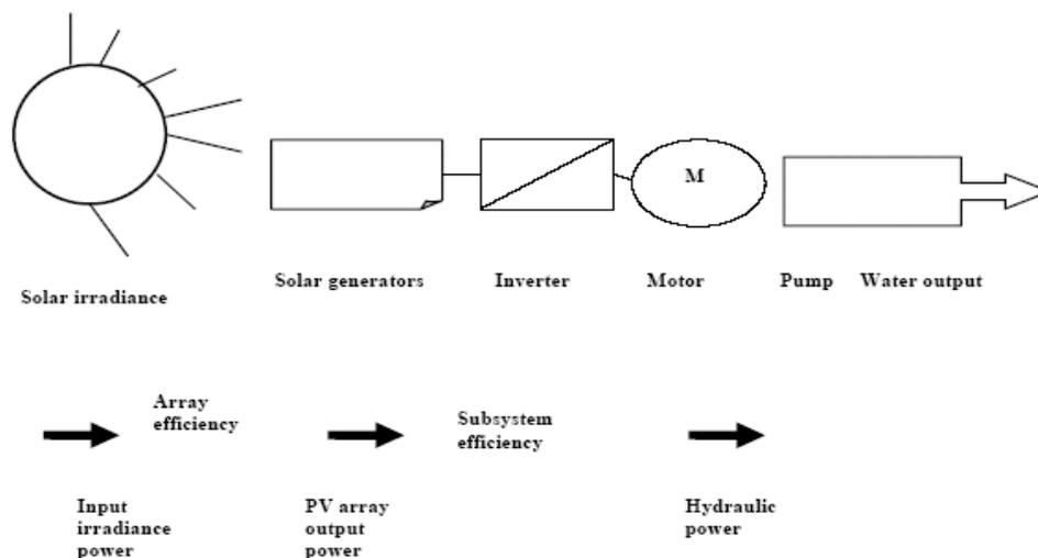
**Figure 1. Solar water pump system.**
