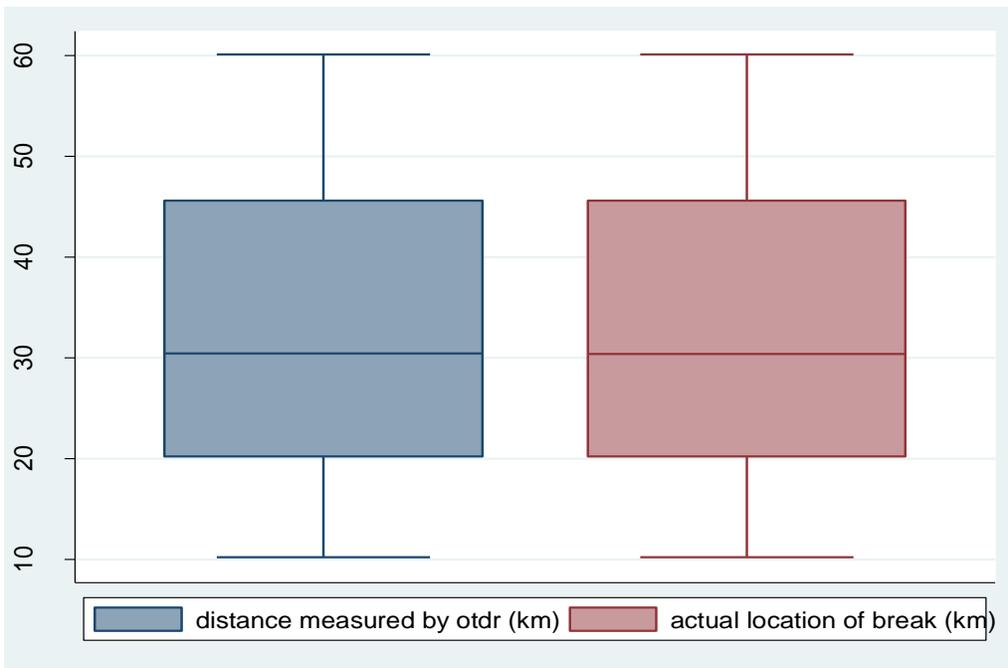
Figure 6: Box plot of distance measured by OTDR and actual location of break from the algorithm
