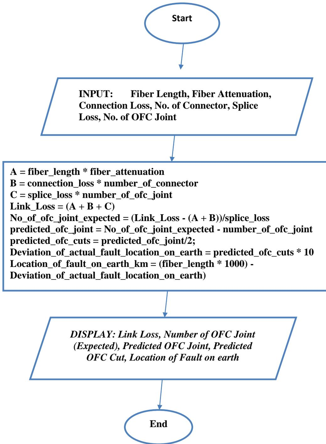
Figure 3: The Flowchart for the Actual Fault Location on Fiber Optic on Earth System
