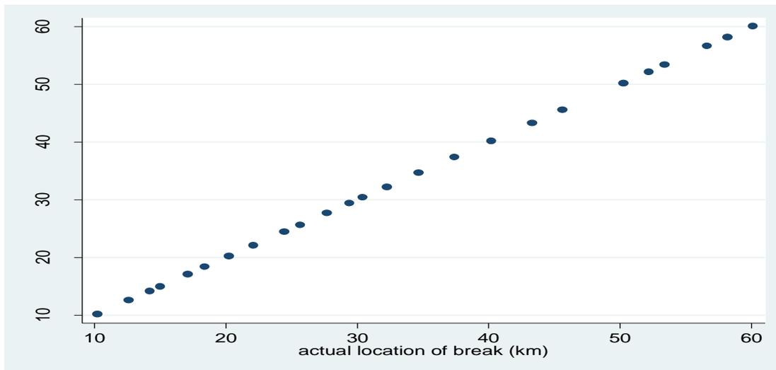
**Figure 7: Distance measured by OTDR against actual location of break from the algorithm**
