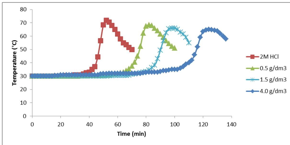
**Fig. 3.** Variation of temperature (°C) with time (min) for aluminium corrosion in 2 M HCl obtained in absence and presence of *Microdesmis puberula* leaf extract
