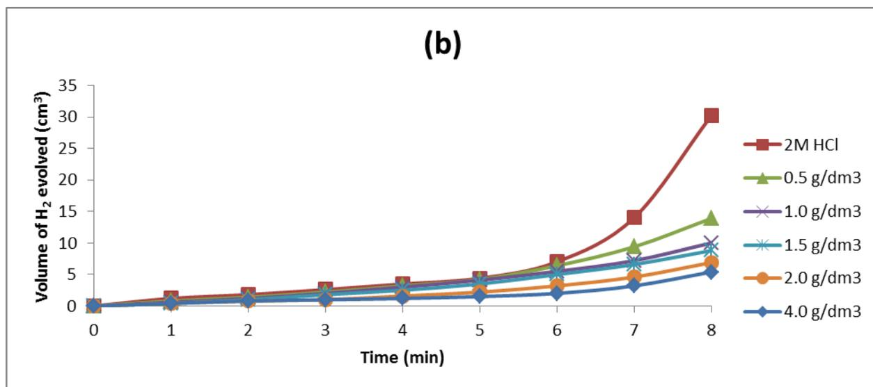
Fig. 1. Variation of volume of hydrogen gas evolved ( $\text{cm}^3$ ) with time (min) for aluminium corrosion in 2 M HCl solution in the absence and presence of *Microdesmis puberula* leaf extract concentrations at (a)  $30^\circ\text{C}$  and (b)  $50^\circ\text{C}$
