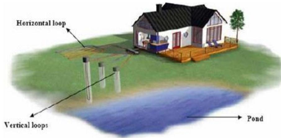
Figure 1. Using the soil, bedrock or groundwater as the heat source.
