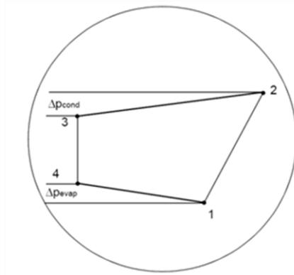
Figure 18. Pressure drops in evaporator and condenser.
