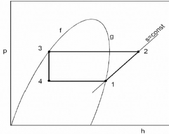
Figure 14. Refrigeration cycle.
