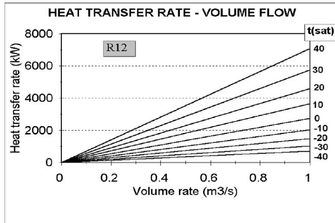
Figure 5. Heat transfer rate versus volume rate.
