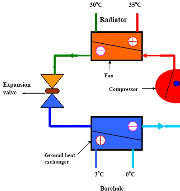
Figure 2. Detail of the GSHP circuit.
