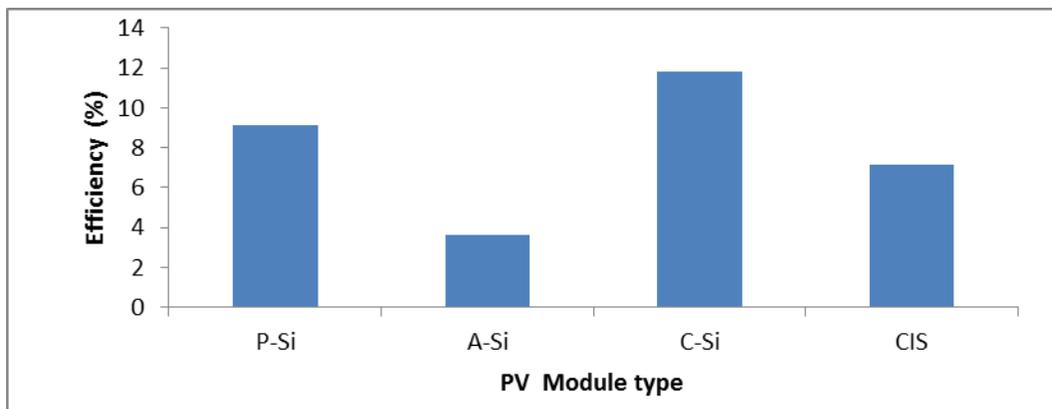
**Figure 3.4: Average module efficiency of each PV module type used in the field study**
