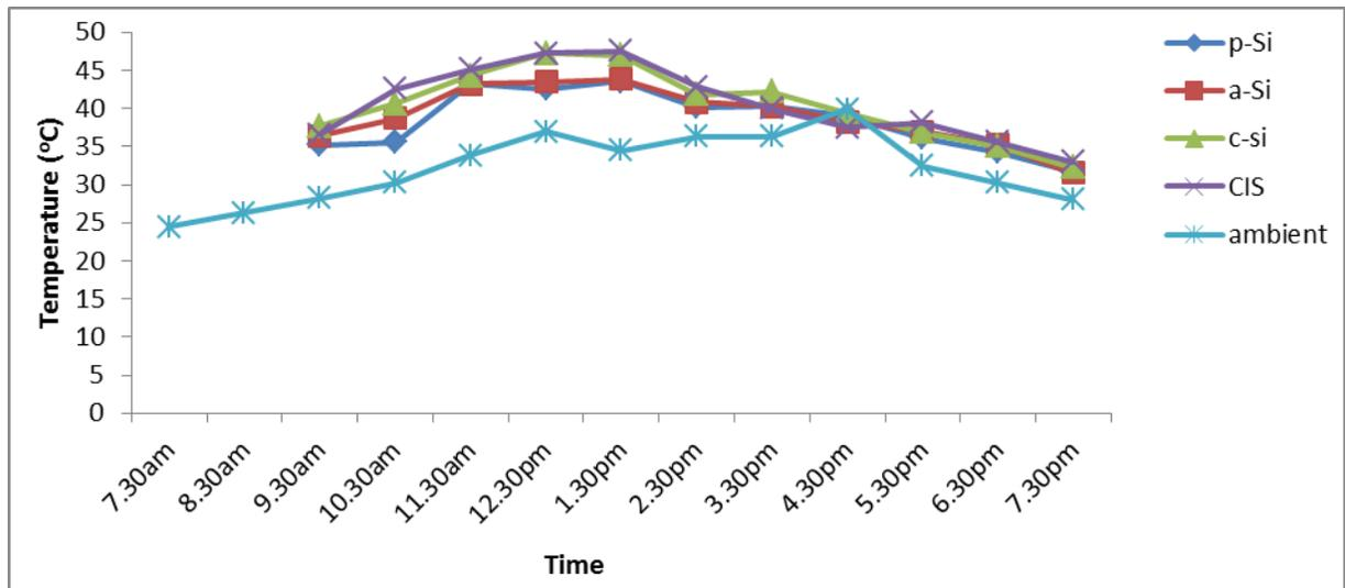
Figure 3.7: Line plot of hourly average ambient temperature versus all the PV module temperatures.
