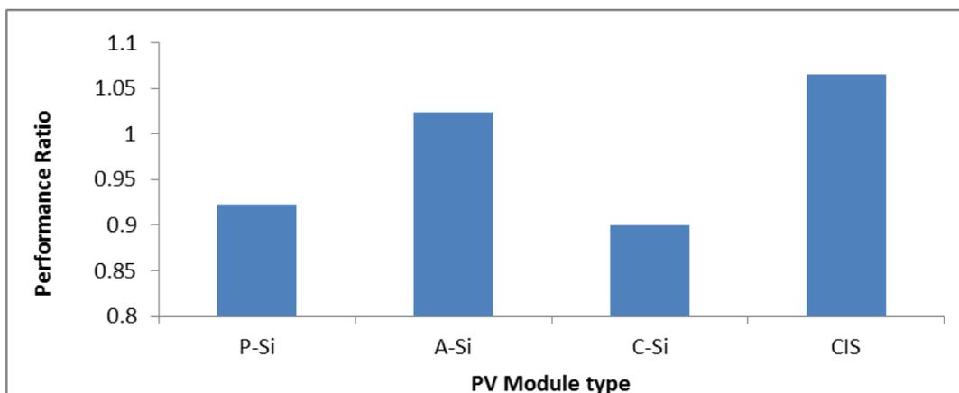
**Figure 3.5: Average performance ratio of each PV module type used in the field study**
