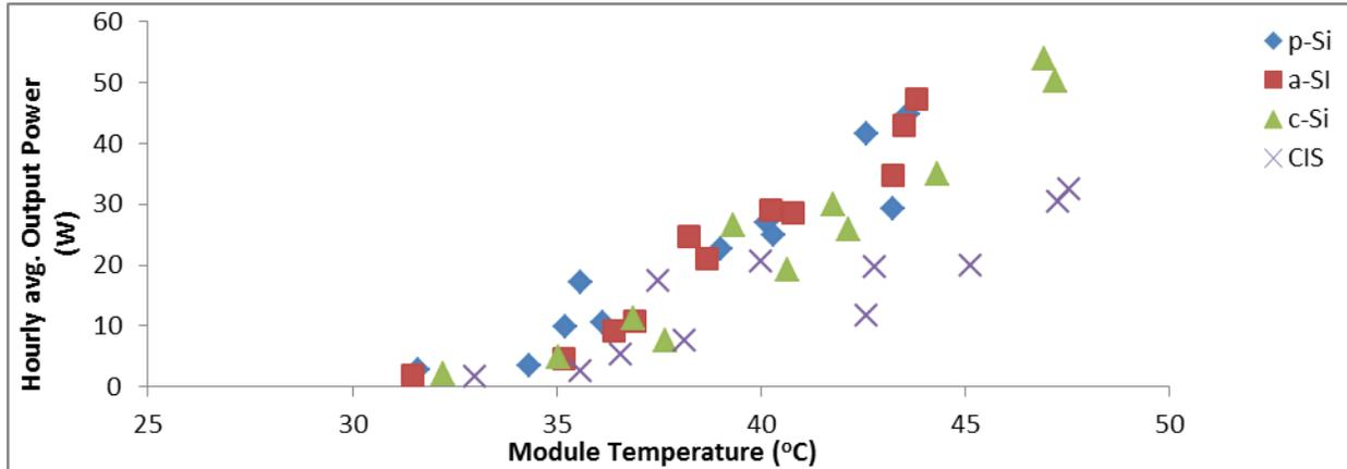
Figure 3.6: Scatter plot of hourly average output power vs module temperature for all the PV modules.
