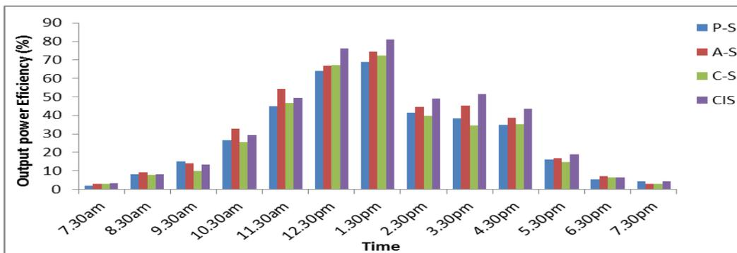
Figure 3.4: Bar chart plot of hourly average of normalized output power efficiency vs time for all the PV modules
