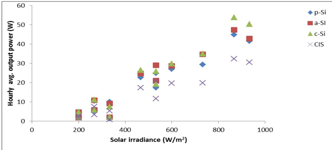
Fig. 3.3: Scatter plot of hourly average output power versus solar irradiance for all the PV modules
