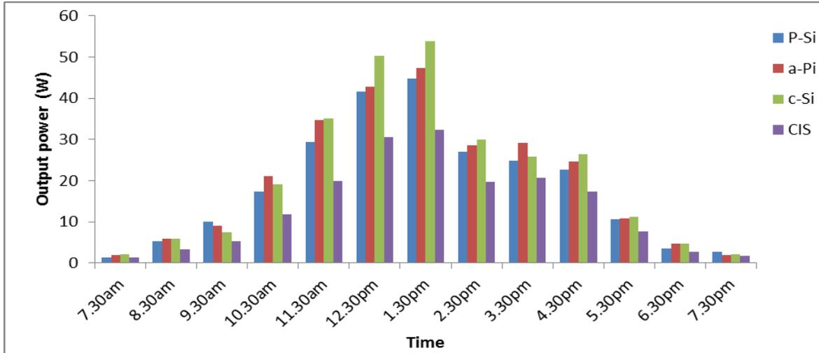
**Fig. 3.1:** Bar chart plot of hourly average output power versus time for all the PV modules.
