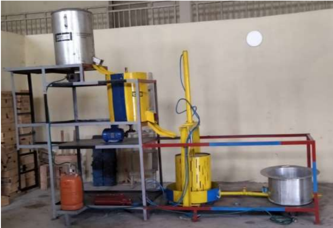
Figure 1: Image of gas powered palm oil processing mill.
