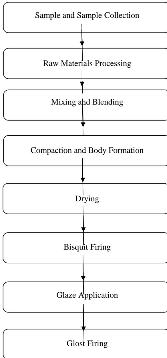
**Figure 1** Experimental steps in the production of ceramics products
