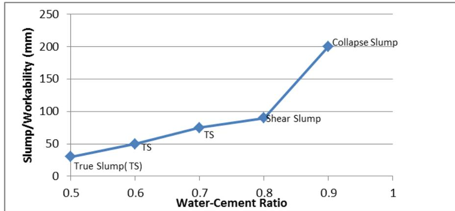
**Figure 4: Workability vs. W/C for Fresh Concrete Mix**
