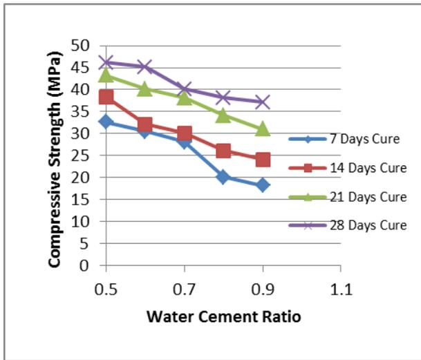
**Figure 1: Compressive Strength vs. W/C for Various Cure Days of Concrete**
