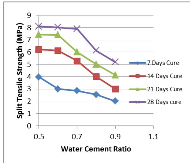
**Figure 2: Split Tensile Strength vs. W/C for Various Cure Days of Concrete**
