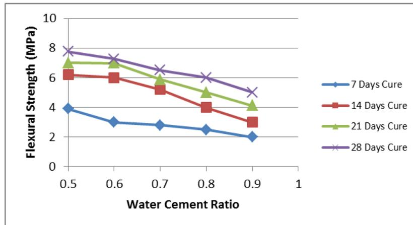
Figure 3: Flexural Strength vs. W/C for Various Cure Days of Concrete
