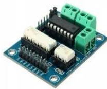
Fig.5 L293D Motor Driver
