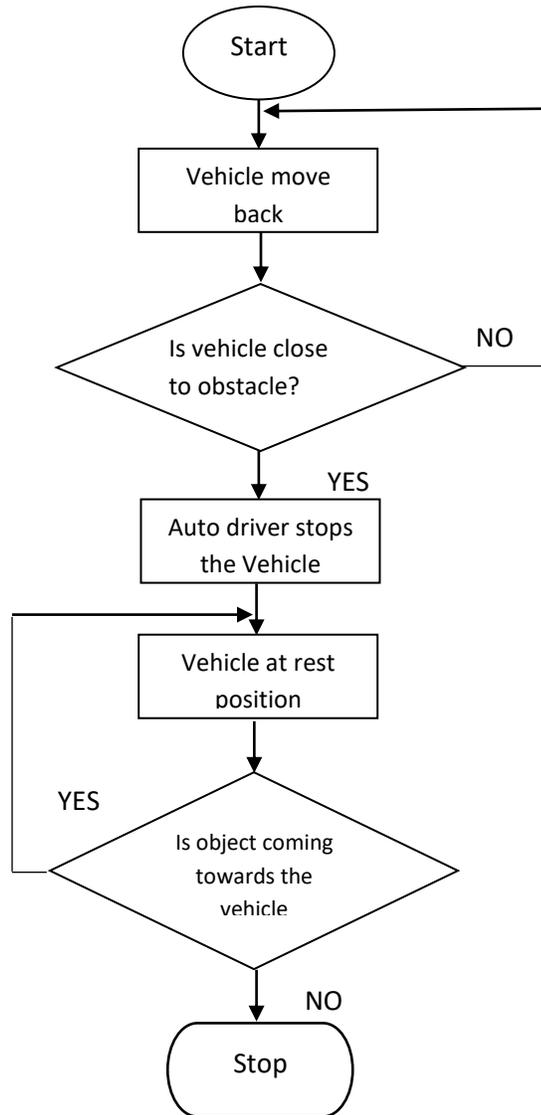
Fig.8 Obstacle detection and avoidance using proximity sensor.
