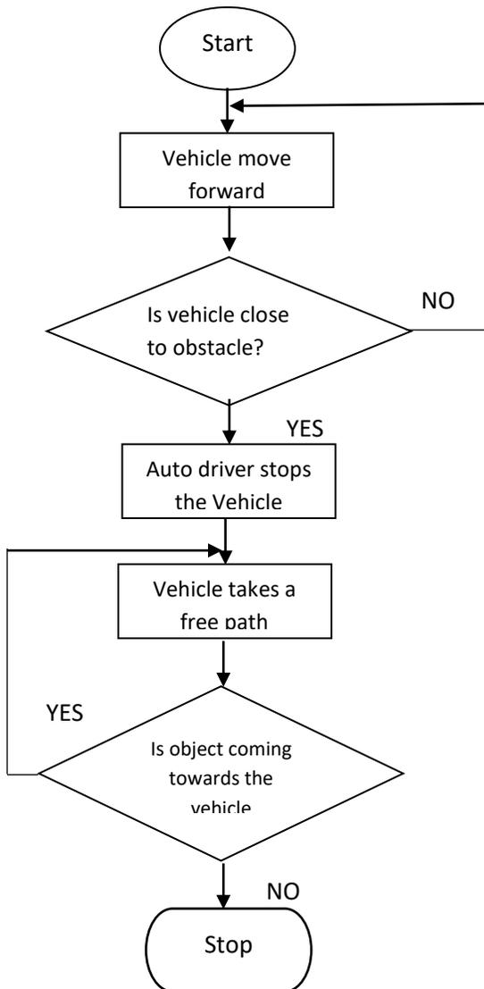
Fig.7 Obstacle detection and avoidance using Ultrasonic sensor.
