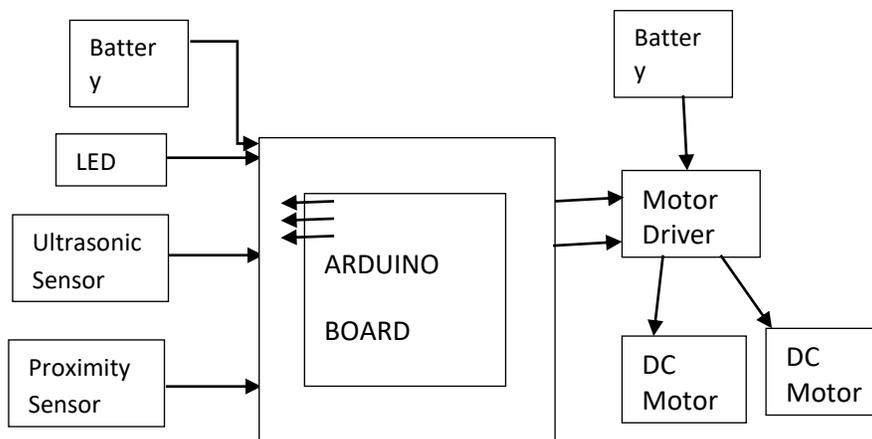
Fig.1 Circuit diagram for the sensors using Arduino controller
