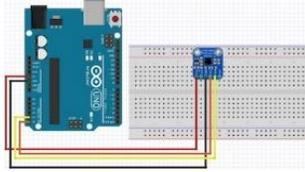
Fig.4 VCNL4010 Proximity Sensor and Arduino Interface Connection
