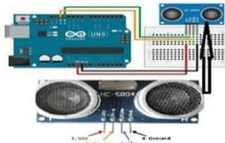
Fig. 3 HC-SR04 Ultrasonic Sensor and Arduino Interface Connection
