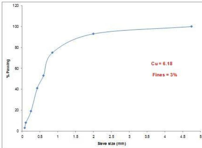
Figure 1: Particle size distribution curve and coefficient of uniformity value for fine aggregate used for the concrete production (Cu = 3; Fines = 6.18).
