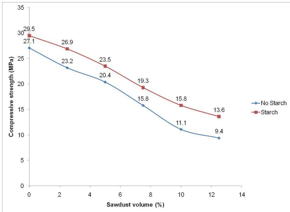
Figure 2: The compressive strength of the concrete at curing day 28
