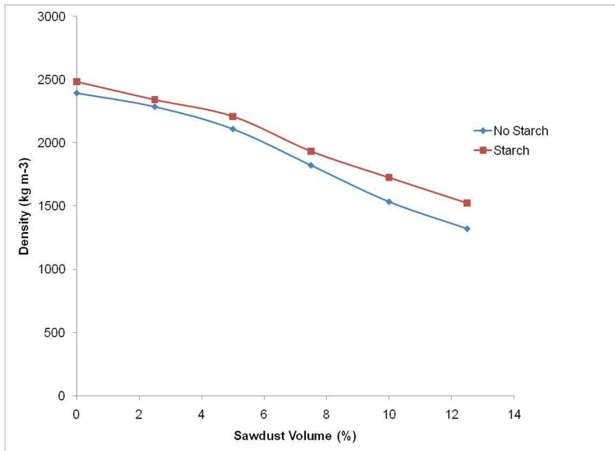
Figure 3: The concrete density at curing day 28
