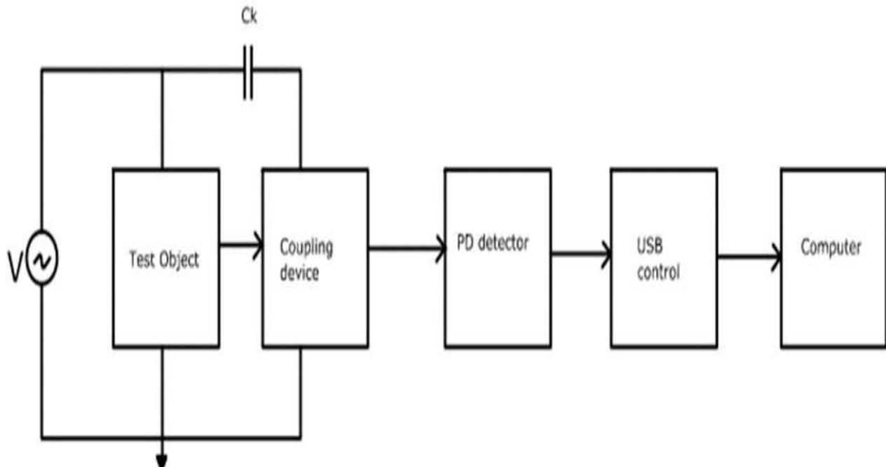
**Figure 3.1: Block Diagram of PD Testing Procedure**
