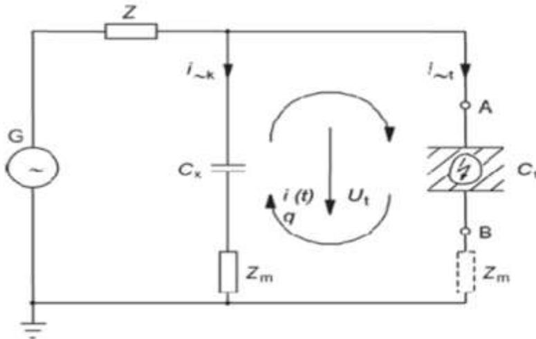
**Figure 3.2: Equivalent Circuit for PD Measurement**
