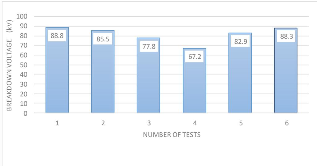
Figure 4.3: Breakdown Voltage Level (kV) at 35°C
