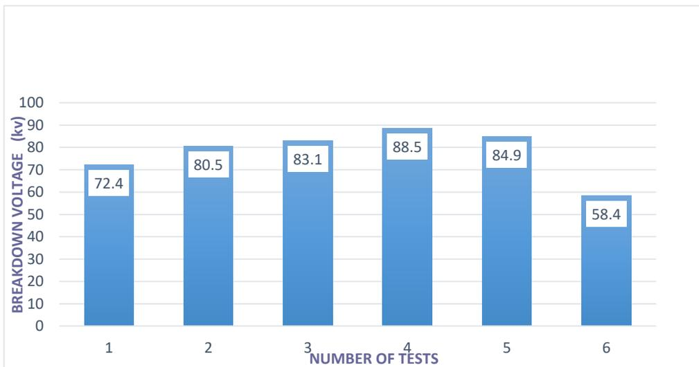
**Figure 4.2: Breakdown Voltage Level (kV) at 34°C**
