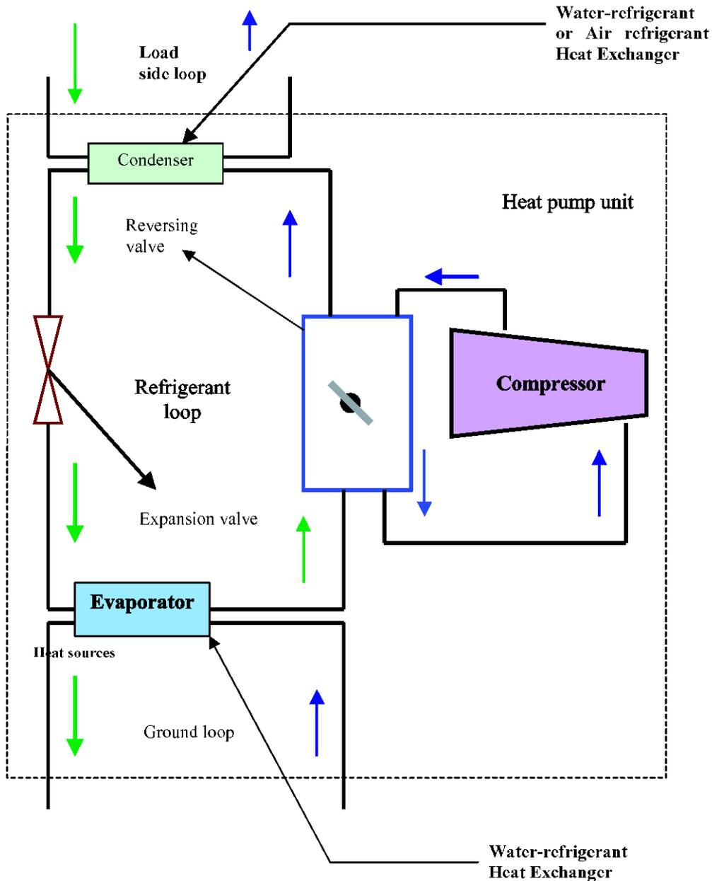
**Figure 8 Schematic of GSHP system (heating mode operation)**
