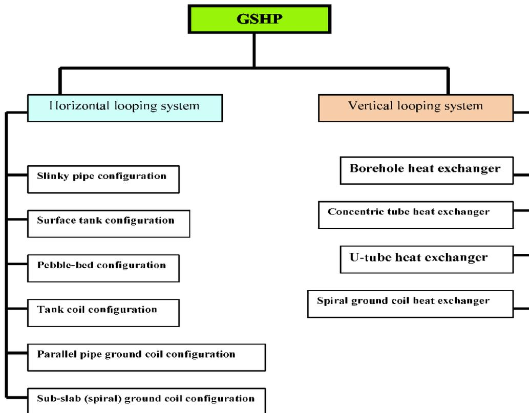
**Figure 7 Common types of ground-loop heat exchangers**
