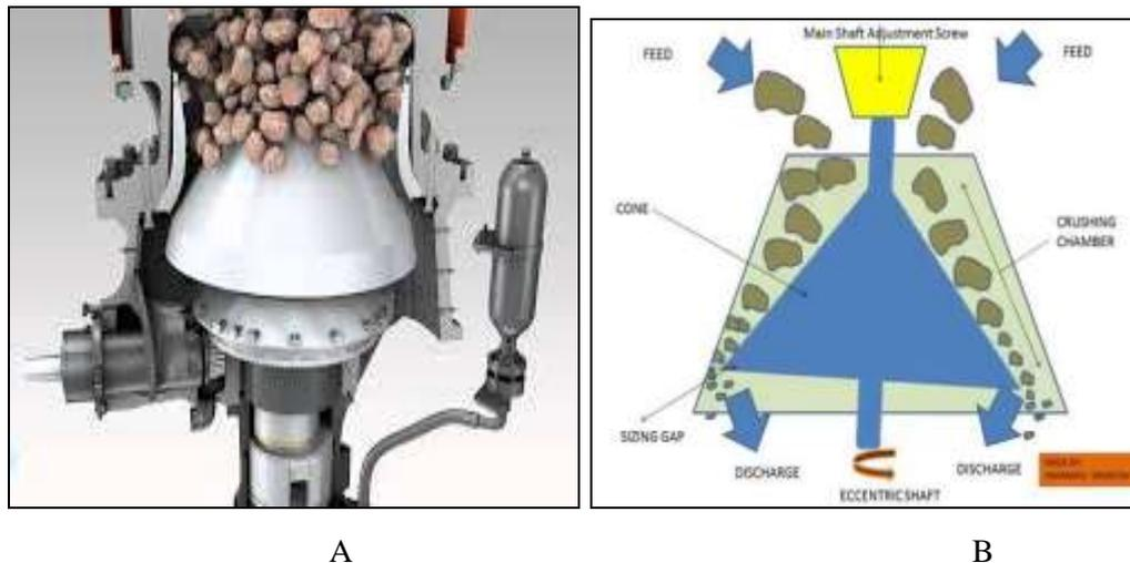
**Fig 5: A Cone Crusher (A) and schematic diagram of a cone crusher (B) (After Thangevelu and Adhikari, 2017)**
