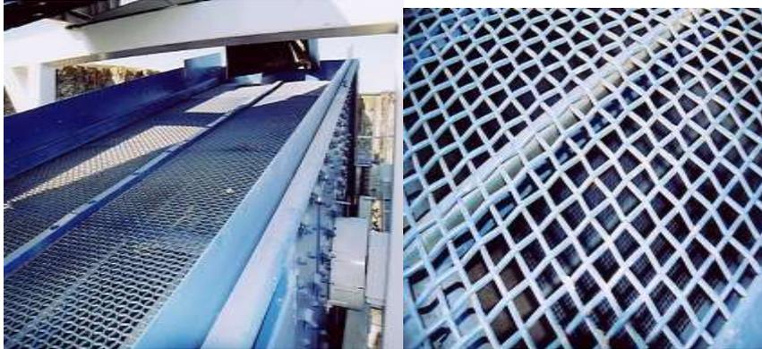
**Fig 6: (A) Triple deck screen. (B) Woven wire screen mesh (www.vibratorscreenmesh.com)**
