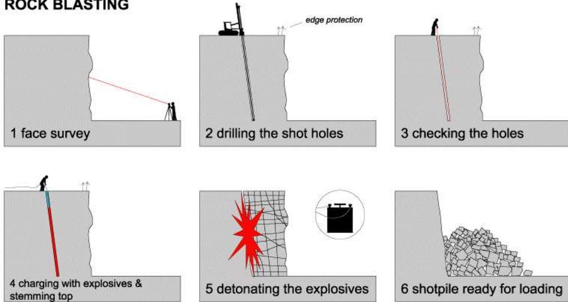
**Fig 4: Schematic description of the blasting process**
