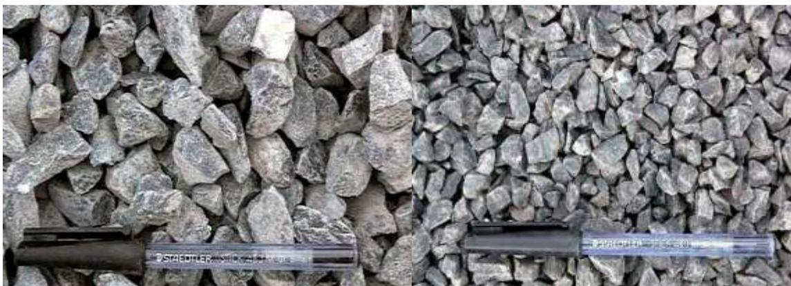
**Fig 7: Screening sizes (A) 14/20 screenings (B) 6.3/10 screenings (ASTM, 2000)**
