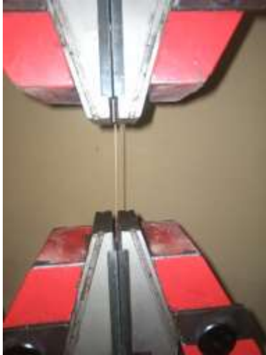
Figure 1: Testing the tensile properties of the cable core with UTM
