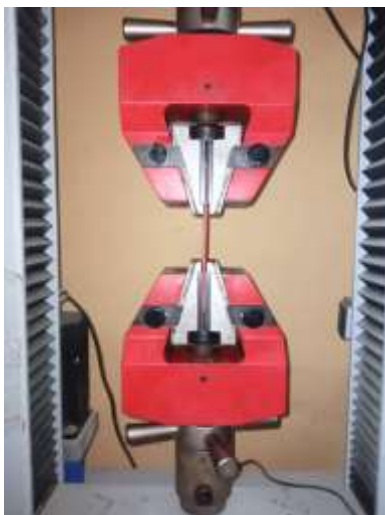
Figure 2: Testing the tensile properties of the cable insulating material with the UTM
