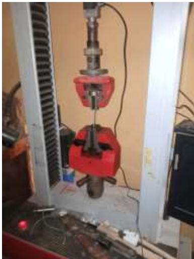
Figure 1: The composite undergoing tensile test
