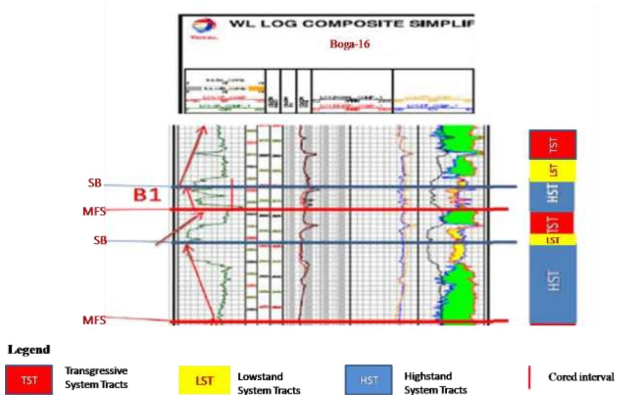
Figure 8: Reservoir “B1” Boga 16 Stacking Pattern and Sequence Stratigraphic Frame work
