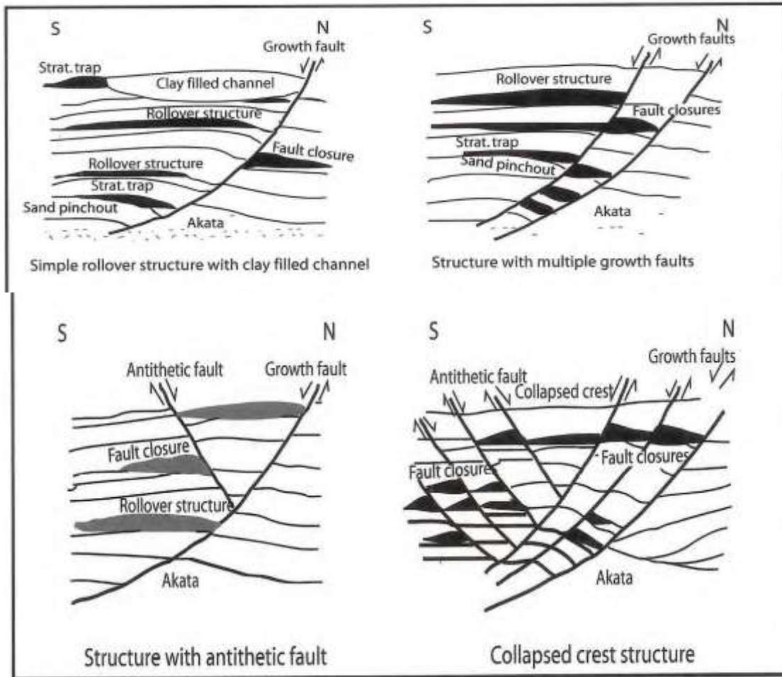
**Figure 4: Examples of Niger delta oil field structures and associated trap types (Burke, 1972; Reijers, et al., 1997; Tuttle, et al., 1999).**
