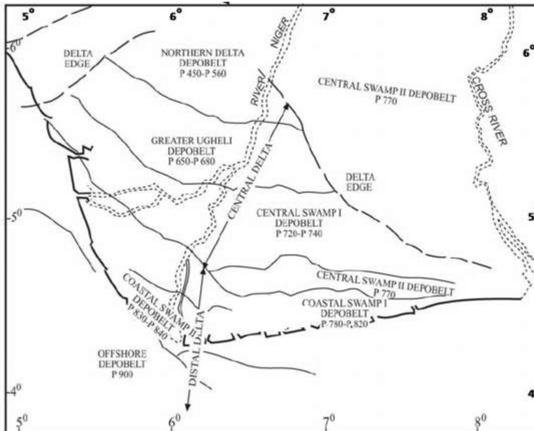
Figure 3: Map of Niger Delta showing the different depobelt (modified after Knox and Omotsola, 1989)
