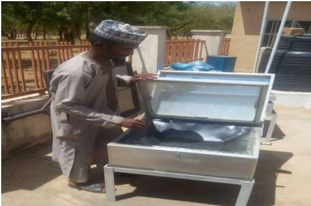
Fig.1b: Outer and inner view of the solar box cooker
