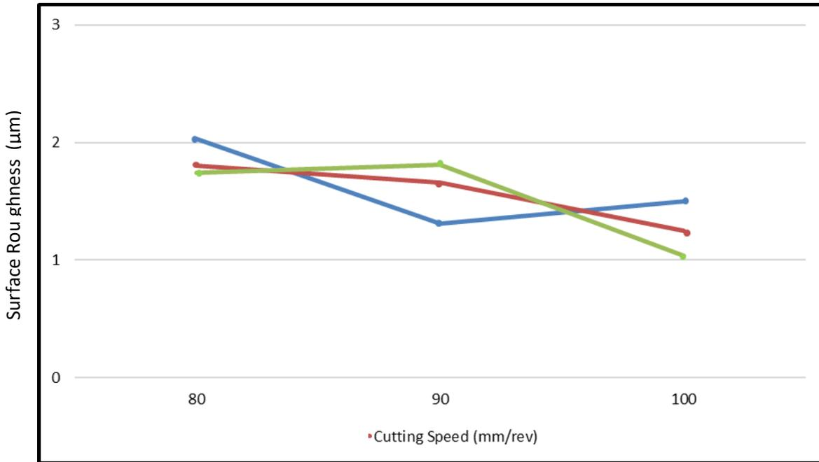
*Fig 1: Average Surface roughness vs Cutting speed*
