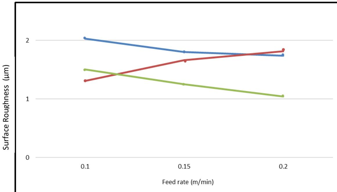
Fig 2: Average Surface roughness vs Feed rate
